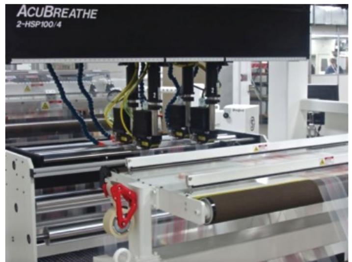
**FIGURE 3.** A multi-head, machine-direction laser micro-perforation station integrated to a slitter/rewinder system. The four laser heads are placing four rows of micro-perforations in the down-web direction at different locations across the web.
