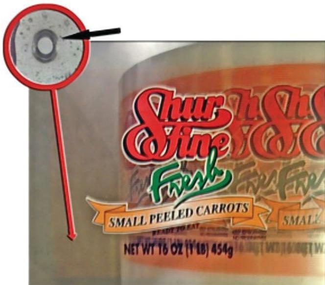
**FIGURE 1.** Machine-direction laser micro-perforating is set up to produce 0.004-in. (100-micron) diameter holes. The number of micro-perforations per package is determined by the OTR required for the produce to be packaged.
