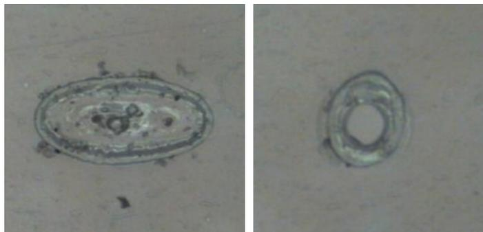
**FIGURE 2.** At a web speed of 1000 fpm (300 mpm), the web will travel 0.020 in. (0.50 mm) during a 100-microsecond laser pulse to produce the micro-perforation. If the focused laser beam remains stationary, the elongated feature (at left) is the result. By incorporating beam compression, where the focused laser beam tracks the web at the same speed, a hole is micro-perforated to specification (right).
